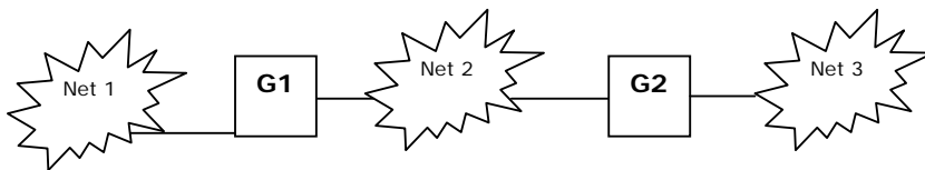
Fig Three networks interconnected by two gateways
